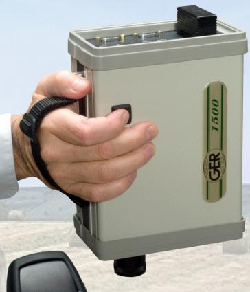
as powering up, selecting the desired foreoptic, integration, and measurement type, then pressing the actuator and aiming the laser. Easing up on the actuator initiates the measurement. Outdoor measurements can be made as quickly as one second in stand-alone mode, reducing the potential for change in solar illumination between reference and target scans.
