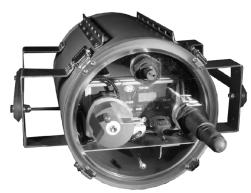
Underwater spectral measurements are acquired using the standard GER 1500 instrument outfitted with the submersible enclosure. Instrument setup is accomplished using the external rotary dial. The laser sight provides targeting guidance. The internal memory can store a day's worth of data and is quickly downloaded without opening the enclosure. The internal battery is designed to provide power for two full days of operation.
